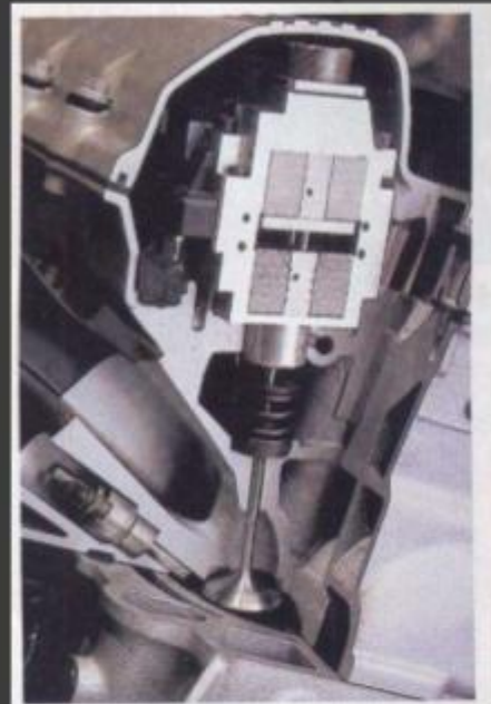
Electronically operated valves could replace cams in the future. This cutaway of a BMW prototype engine shows the powerful solenoid above each valve that controls its movement.
